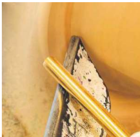
▲ Pic.14 Set the lathe to 1,800rpm for the final finishing cuts. This technique is so much easier at a higher speed, but if you don't feel safe, reduce the speed – this just requires more sanding
